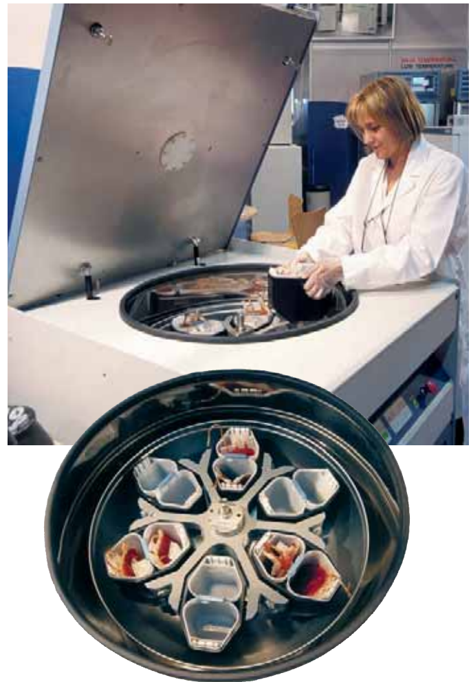
Image showing the rotor and double buckets for quad and triple blood bags of 500 and 800 ml.
